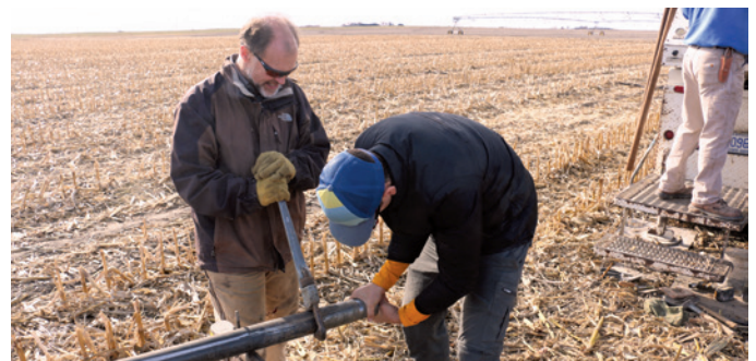
WSL Director Dan Snow and University of Nebraska-Lincoln graduate student Craig Adams prepare a soil core from the vadose zone.
